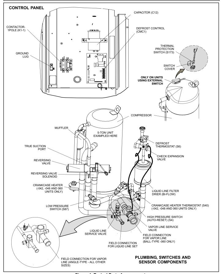
Figure 1. Typical Parts Arrangements
